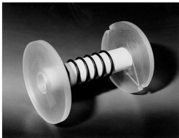
Figure 4 Photograph of the as-extruded Y123 wire with good flexibility, which was wound on to a bobbin.
